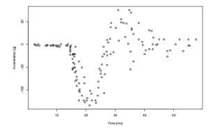
$\bullet$  head acceleration Y depending on time X in a simulated motorcycle accident used to test crash helmets
